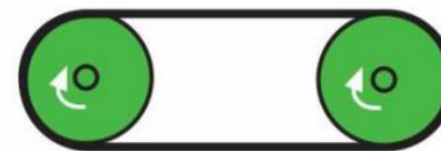
The pulleys rotate in the same direction
